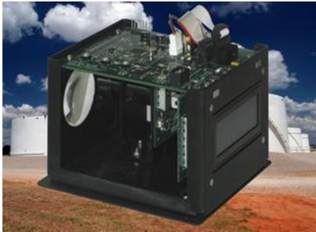
The LLM-100 cage houses all electronics and modules for the LLM to function.
