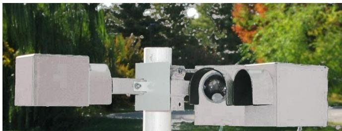
The OWI-650 LP-WIVIS™ has been designed from the ground up for quick deployment anywhere. The LP-WIVIS is the first present weather and visibility sensor designed for battery powered or solar powered applications.
